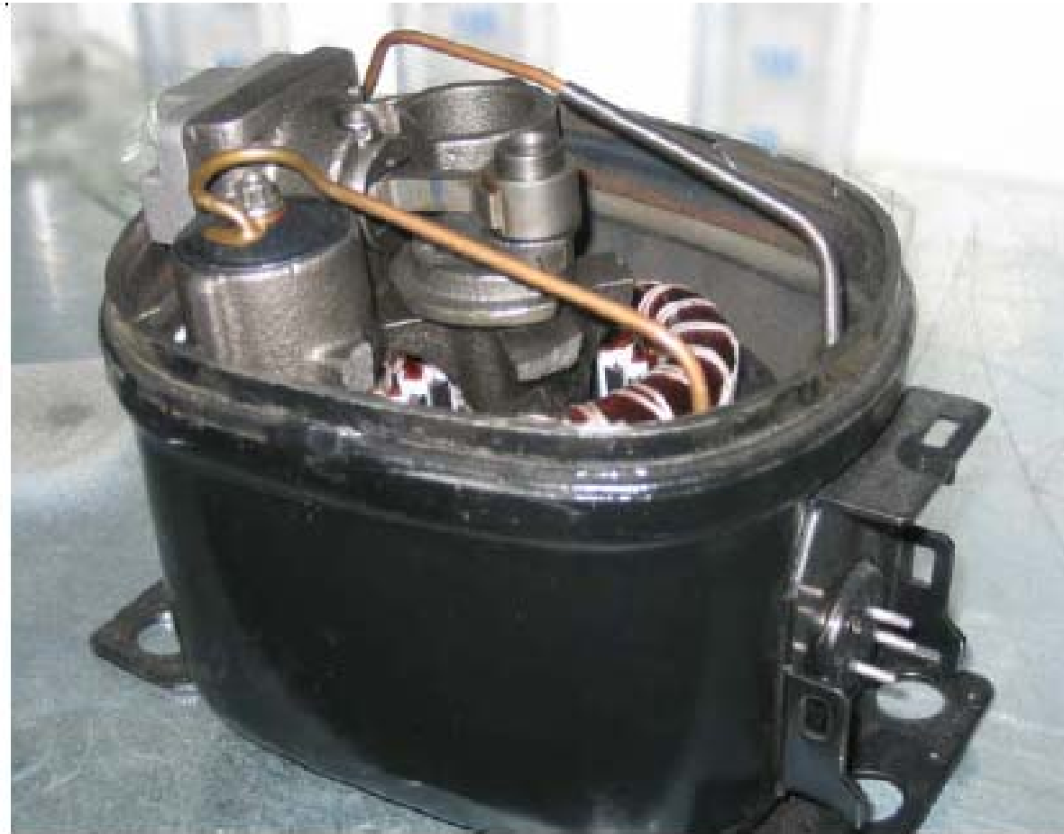
Figure 2: Hermetic piston compressor for household refrigerators with opened shell
