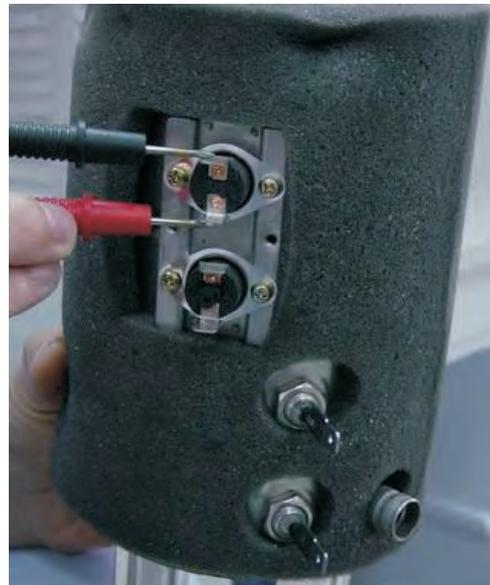
3. Use the multimeter to check the heater. If the heater works, the multimeter will appear data or beep, Contrarily then contrary.
