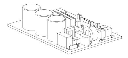
For other models, connect discharge resistance (approx.100 $\Omega$  40W) or a soldering iron plug between the positive and negative terminals of the electrolytic capacitor. The terminals are located on the bottom surface of the outdoor PCB.
