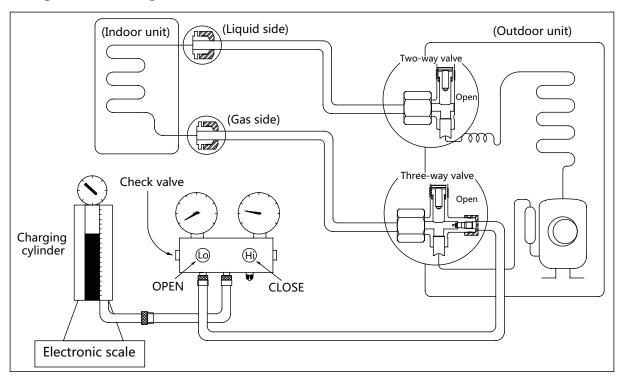
Prior to recharging the refrigerant, confirm the additional amount of refrigerant required using the following table:
