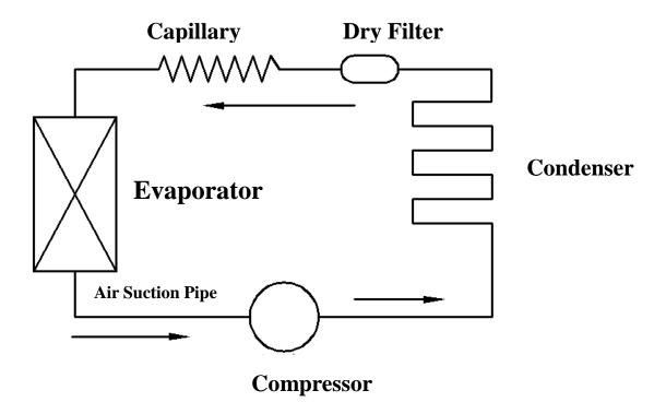
Note: Arrow direction means the flowing direction of the refrigerant.
