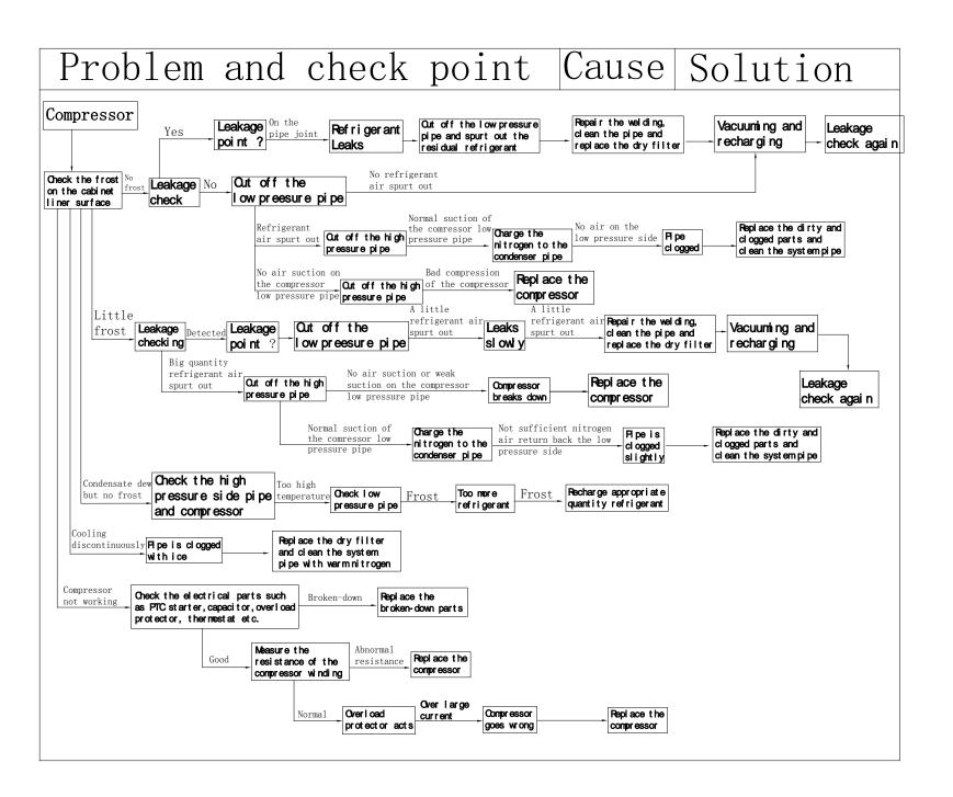
Check the frost on the cabinet liner surface, if find like following:
