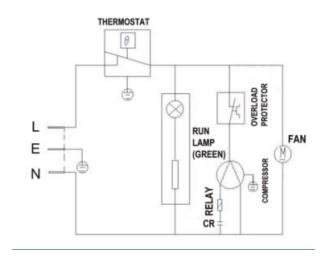
Please note, maybe some units are without RUNNING CAPACITOR marked in red color in above diagram, according to the used compressor model.
