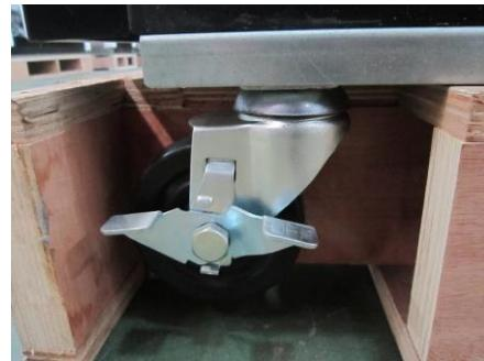
The caster has a brake. Turning it to different sides can lock or unlock the caster.
